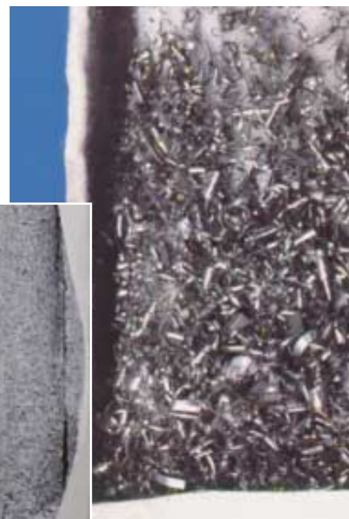
Metal fines collected from parts washer
