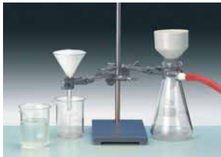
Vacuum filtration using a filter disc in a Buechner funnel (right side). Courtesy of Phywe Systeme GmbH
