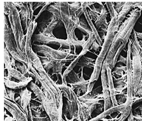
Cross section of a filter paper under a microscope
